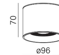
**ONLY round mini LED 230V exterior surface** [aqform.com/ON1974](http://aqform.com/ON1974)
